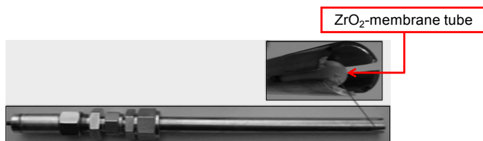
a. High temperature/High pressure ZrO 2 -based pH electrode
